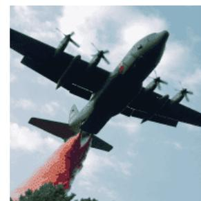
consists of seven airborne modules and one ground air compressor module. The system can be loaded on a C-130 aircraft in two hours, and filled with retardant and compressed air in 15 to 20 minutes. The system is self-contained and requires no aircraft modifications. Each system weighs 10,500 pounds empty, and has a capacity of 2,700 gallons.
